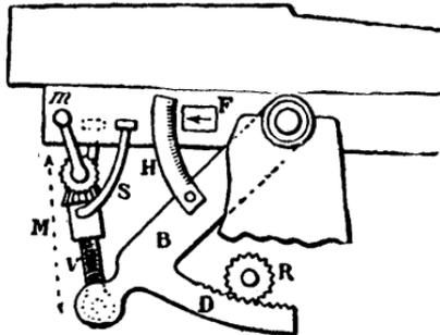
FIG. 5.—Elevating gear.
