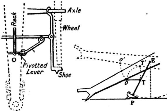
FIG. 3.—Wheel-brake gear.
